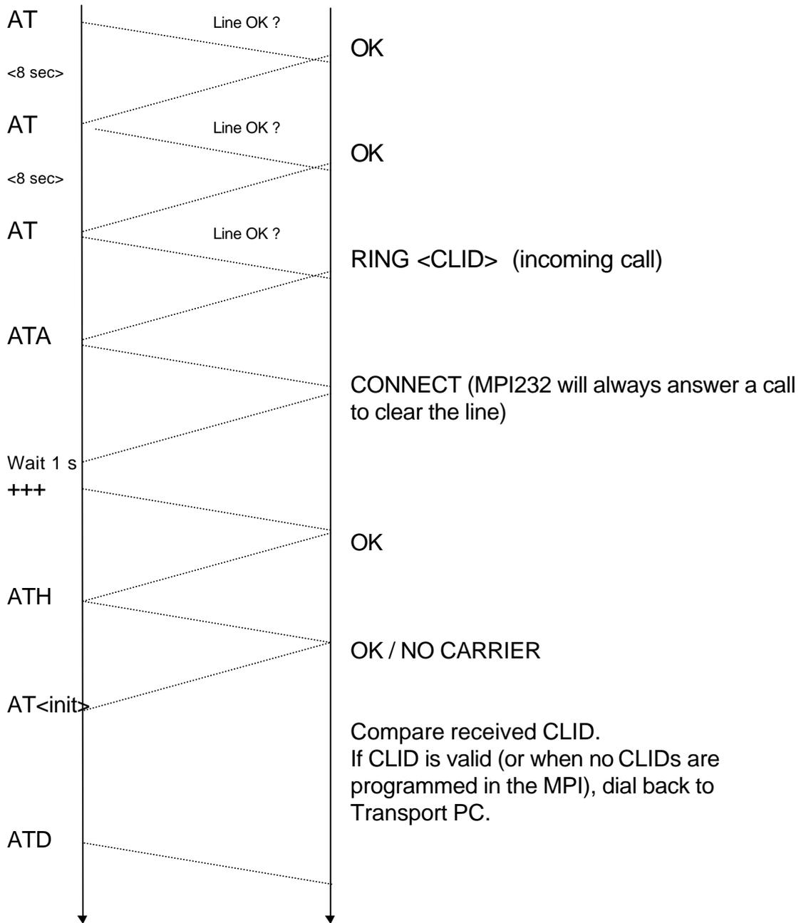
The RING can occur at any moment, and doesn't have to be synchronised with the AT's sent by the MPI. See the attached description of Transport PC for a more detailed description of up-download. If there is one or more CLID strings programmed in the MPI, the received CLID must match one of the programmed strings, otherwise the MPI will not dial back.
