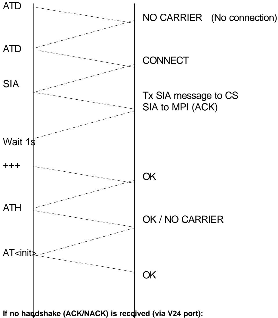
**If no handshake (ACK/NACK) is received (via V24 port):**
