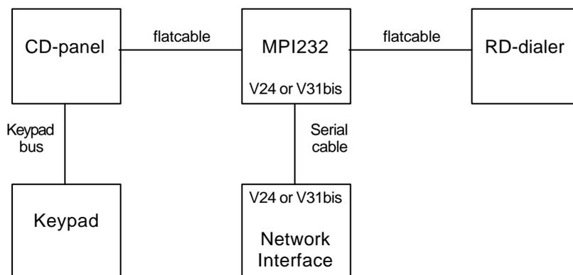
Note that only one serial port of the MPI232 can be used at a time, so the Network Interface will be connected to the V24 (RS232) port or the V31bis (current loop) port.
