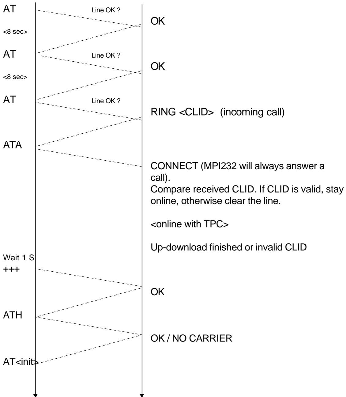
The RING can occur at any moment, and doesn't have to be synchronised with the AT's sent by the MPI. See the attached description of Transport PC for a more detailed description of up-download. If there are no CLID strings programmed in the MPI, the MPI will hang up.
