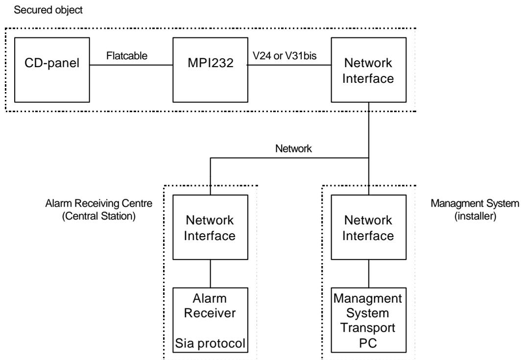
Usually the Alarm Receiver and the Management System are two different systems.
