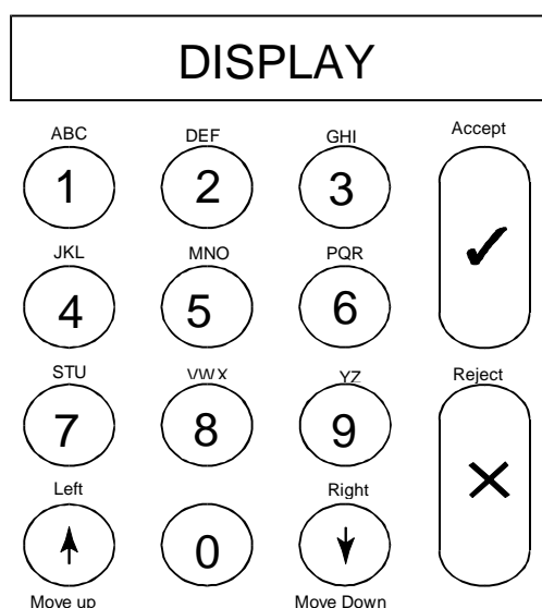
Figure 1. Keypad of the CD30xx
