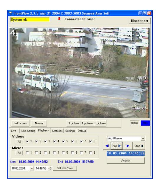
Before the play back can be started, a starting time must be entered. By default, the time of the last recording is used. As an alternative the **Activity representation** can
